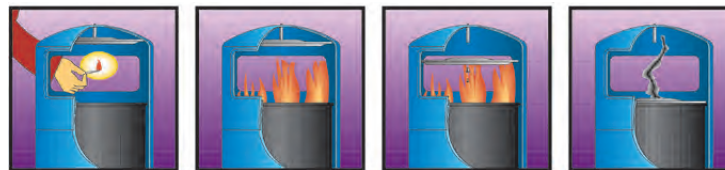
STAGE 1 A burning match is carelessly discarded into a litter bin. STAGE 2 The fire takes hold. STAGE 3 In under a minute, the fire extinguishing plate drops onto the liner. STAGE 4 The fire is contained.
