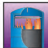
STAGE 3 In under a minute, the fire extinguishing plate drops onto the liner.
